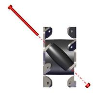
**Step 5:** Tighten all M3-0.5 X 45mm Socket Head Screws and M3 Nylock Nuts to lock all the wheel components in place.
